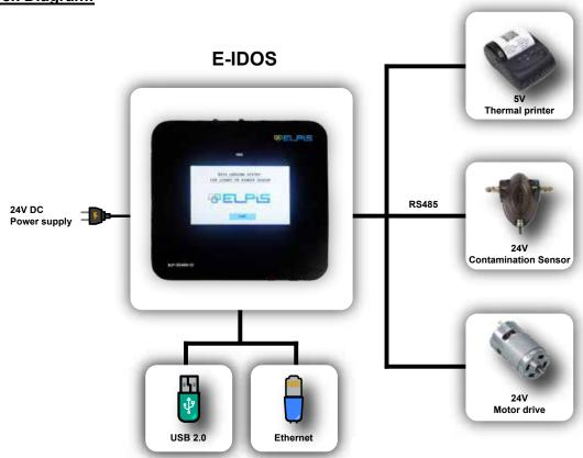
\*DAQ HMI interfaces with external components like thermal printer, contamination sensor and motor.
